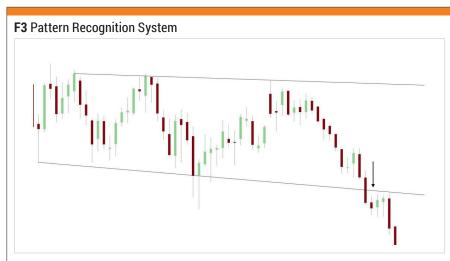
The figure shows a simplified example of how the algorithm recognizes a trend channel and generates a signal based on it (see arrow).
